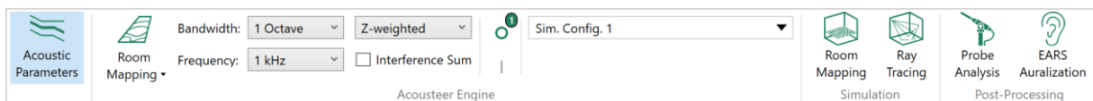
Figure 12.1 Calculations ribbon menu offering access to mapping, ray-tracing, post-processing and auralization functions.
